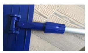
4. To lengthen the handle hold the lower part firm and turn top part anti-clockwise. Extend handle. Hold lower part firmly and turn the upper part clockwise to tighten
